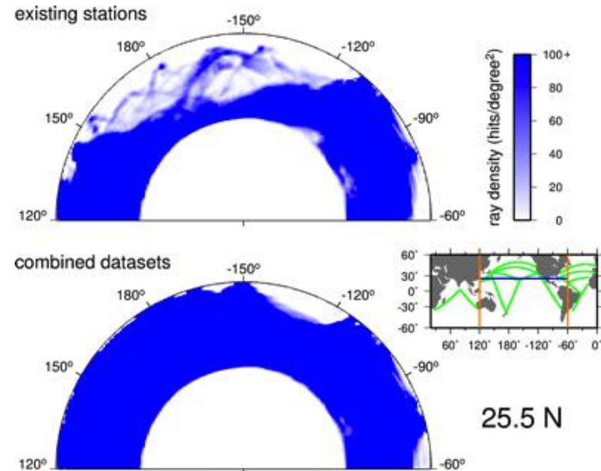
Additional sampling with SMART cables in Pacific, 20 y earthquake sources
