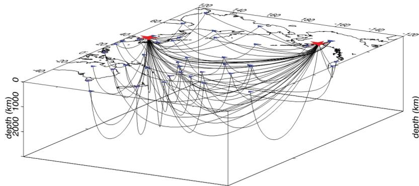
Rays to SMART Cable sensors provide improved coverage over large areas.
